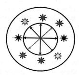
Whenever tyres are replaced on the bus due to issue of new tyres, replacement of punctured tyres, tyre rotation etc.,, the same shall be recorded in shift RG register and given as BF for next day also, to tighten the wheel nuts as is done in case of tightening the spring assembly U-clamp nuts. Tightening on the second day shall be ensured by the shift supervisors and certify the same in a separate register maintained with bus numbers, dates of fitment and tightening.
